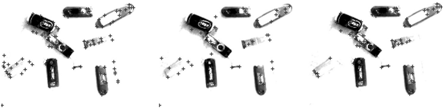
Figure 7-7. Machine corner detection using the Shi-Tomasi method marked with crosses; results are shown using different parameter settings and thresholds for the strength and pixel size of the corners
